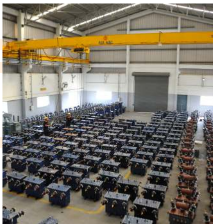
Material handling capacity up to 300 MT
