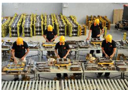
Core Building for Distribution Transformers
