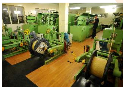
Paper Wrapping on Conductor
