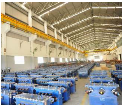
Distribution Transformer Assembly Line
