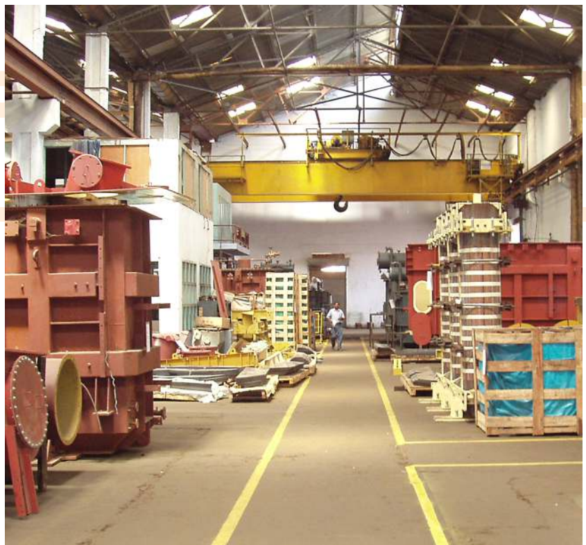
Material Handling facility up to 300 MT
